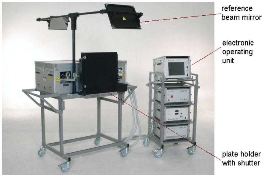
**Figure 5.1:** The latest generation of holographic cameras is mobile: It fits into boxes that may be transported in a car. The hologram plate is put behind a shutter, so the recording works at any ambient light condition.
