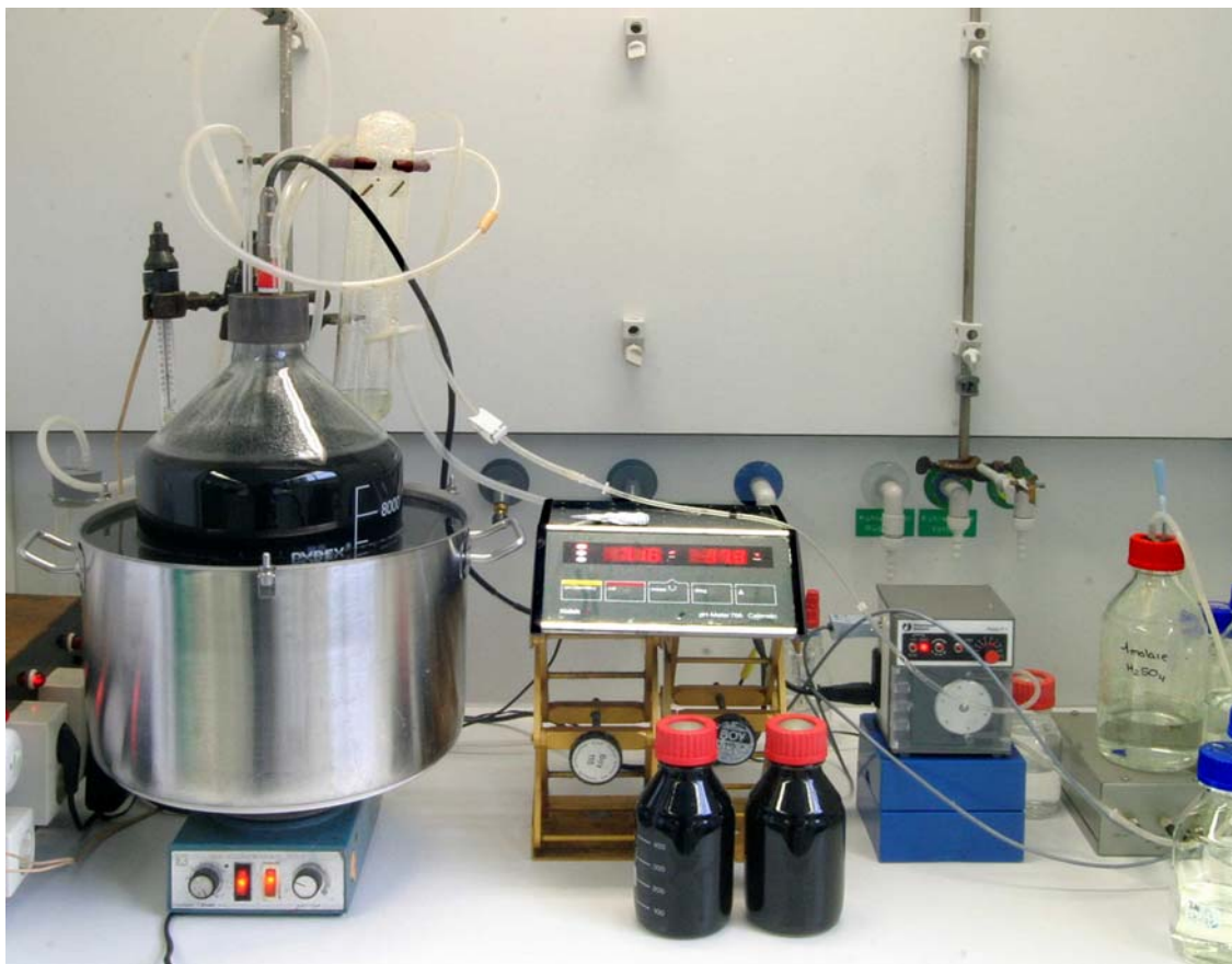
Fig. 3.1 Home built 10-litre glass fermentor. Water bath is used to maintain the temperature at 37°C. pH is maintained in a range of 7.0-7.4, with 1M H 2 SO 4 connected via a manually controlled pump. Fermentor is maintained anaerobic by bubbling with N 2 . Inoculum is added through the same pump as for acid.
