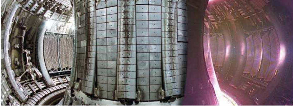
Figure 5.1: The inside of the JET tokamak with (right) and without (left) plasma. Photo: EFDA-JET.
