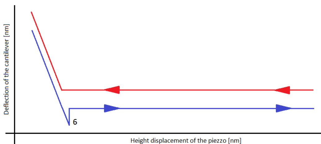
Figure 6-5: Force curve of a small molecule detaching at an early point.
