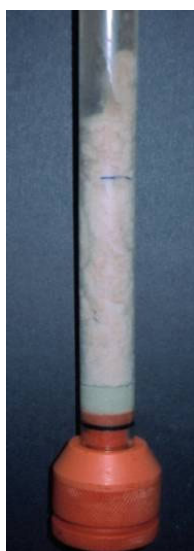
Fig. 6-31: Streamline DEAE after application of Escherichia coli bead mill homogenate
