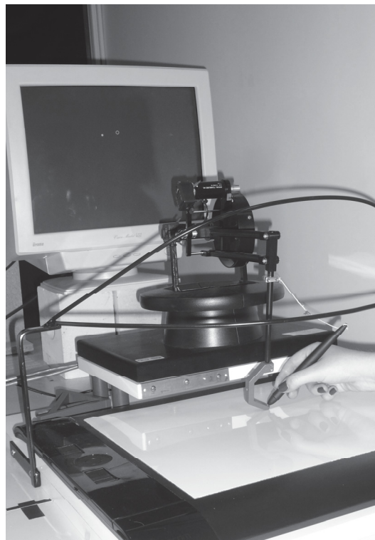
Fig. 1 Apparatus: Participants were seated in front of a digitizer tablet and faced a monitor. The tip of the pen was attached to the lower end of the stylus of a Phantom 1.5.
