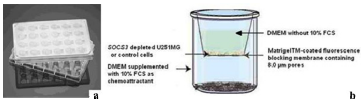
Figure 12a and 12b: This figure shows the principle of modified Boyden chamber assay. 24well; BD Biosciences, San Jose, CA. (modified from URL: http://www.bioscience.org/ ).
