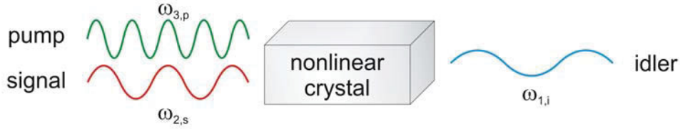
Figure 4.2 Simplified principle of the difference frequency generation (DFG) in a nonlinear crystal.
