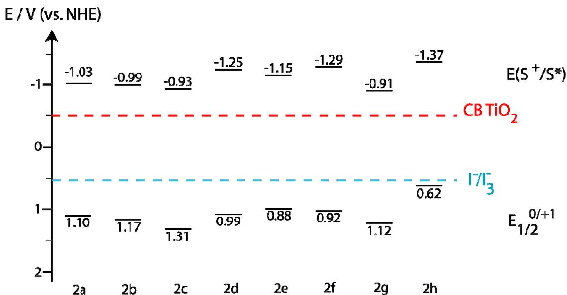
Figure 4. Schematic energy level diagram (HOMO – LUMO) for the dyes **2a-h**.
