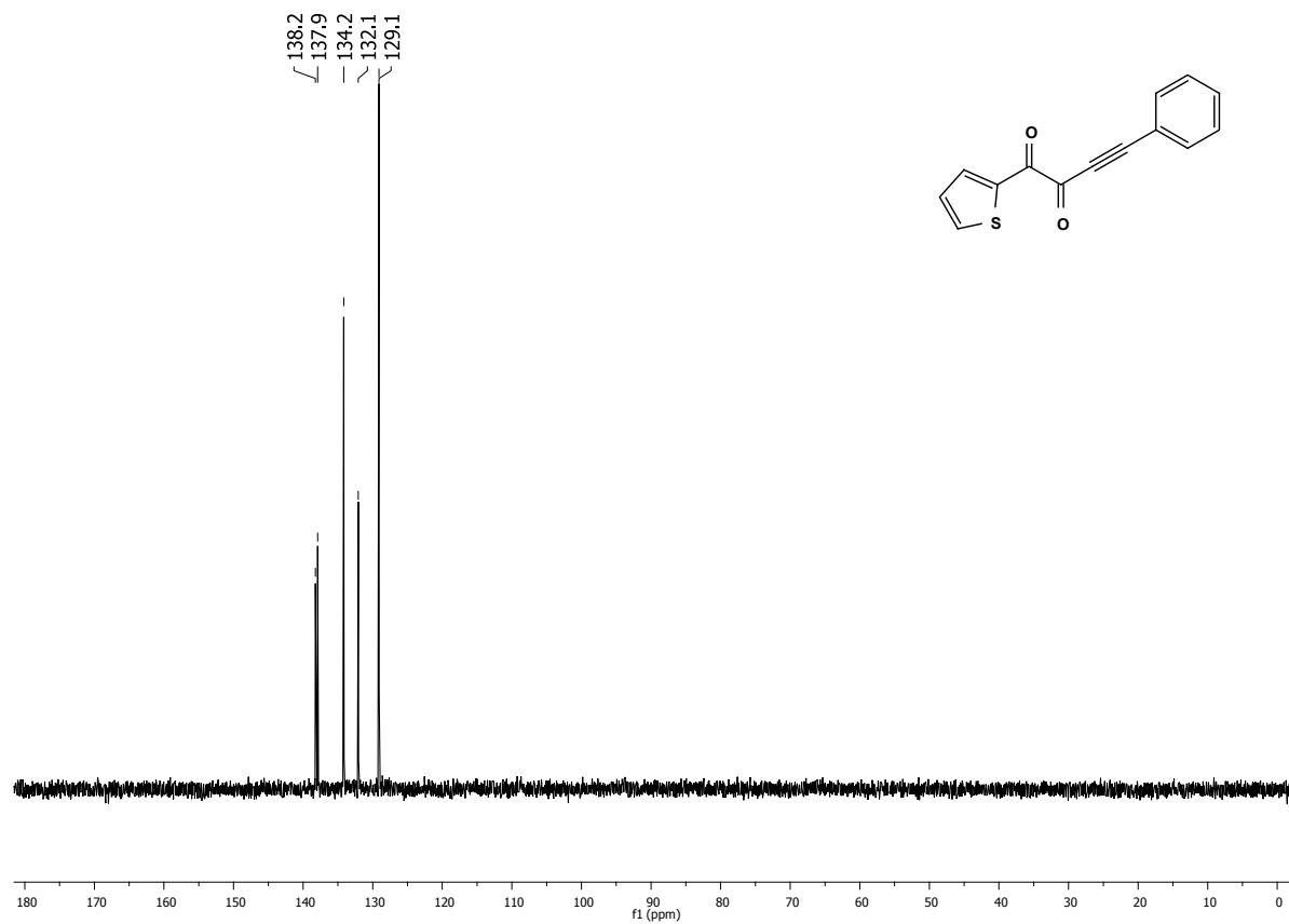
13 C-DEPT 135-NMR (75 MHz) of 3d (30 mg) in CDCl 3 at 296 K ( \delta in ppm).
