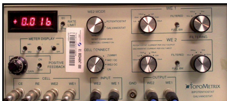
Fig.(3-7): The Topometrix bipotentiostat used in the EC-STM experiments.
