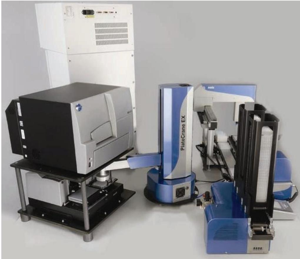
**Figure 3: A fully automated high throughput screening setup. The readout includes fluorescence intensity and polarization, luminescence and ELISAs**
