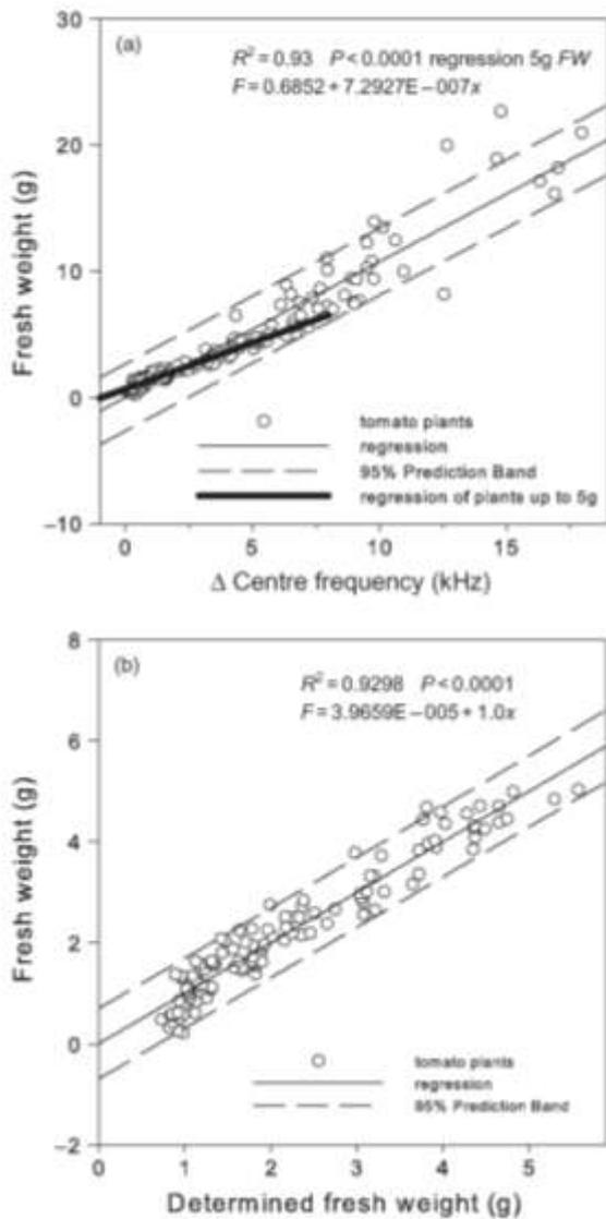
**Figure 5.** Calibration and testing of tomato fresh weight determination. (a) Calibration of the  $\Delta CF$  signal for shoots up to 22 g of fresh weight. (b) Comparison between determined fresh weight calculated from linear regression (up to 5 g, see Fig. 5a) and balance-measured fresh weight.
