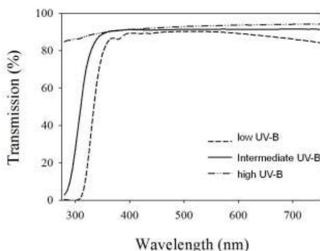
**Figure 1:** Transmission spectra of Float glass (low), MM glass (intermediate) and ETFE foil (high UV-B transmittance) from 280 to 750 nm, measured with a UV/Vis spectrophotometer
