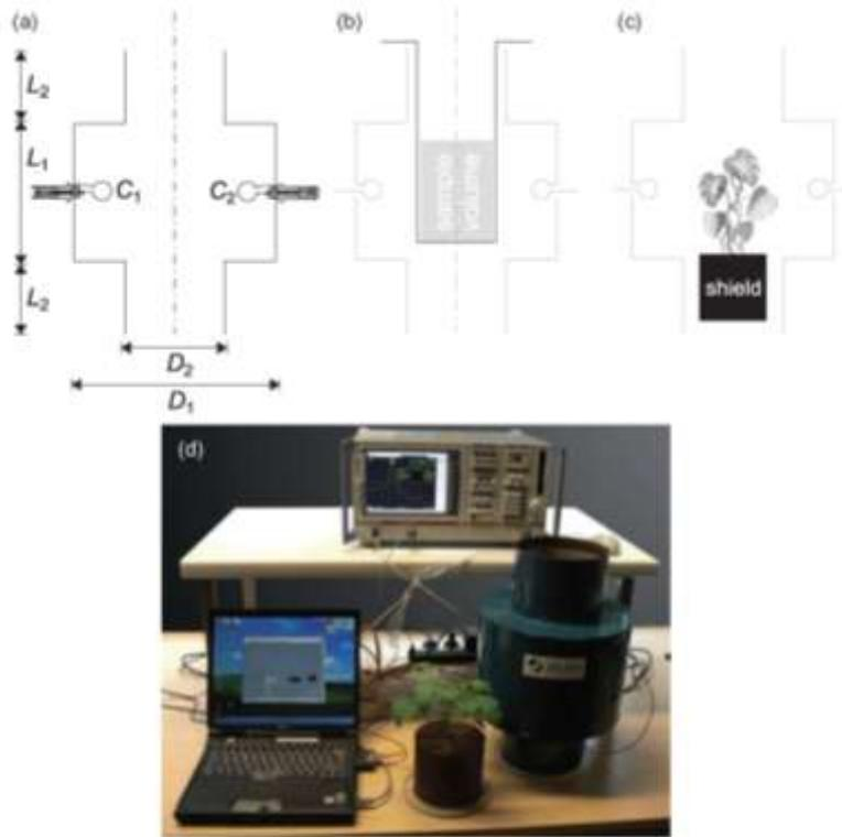
**Figure 1.** Design of the microwave resonator set-up. (a) Schematic of a resonator with dimensions  $D_1$ ,  $D_2$ ,  $L_1$  and  $L_2$  listed in Table 1. (b) Schematic of the Perspex-container for water calibration and cut shoots measurement. (c) Schematic of the copper shield positioning, containing a pot with intact plant. (d) Photo of the measurement setup; top, network analyser; bottom, measurement computer, tomato plant with copper shield and microwave cavity resonator.
