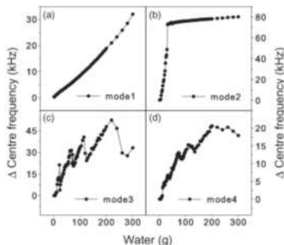
**Figure 3.** Correlations between water content and corresponding delta centre frequencies ( $\Delta CF$ ) for first to fourth microwave resonator mode in panels a, b, c and d, respectively.
