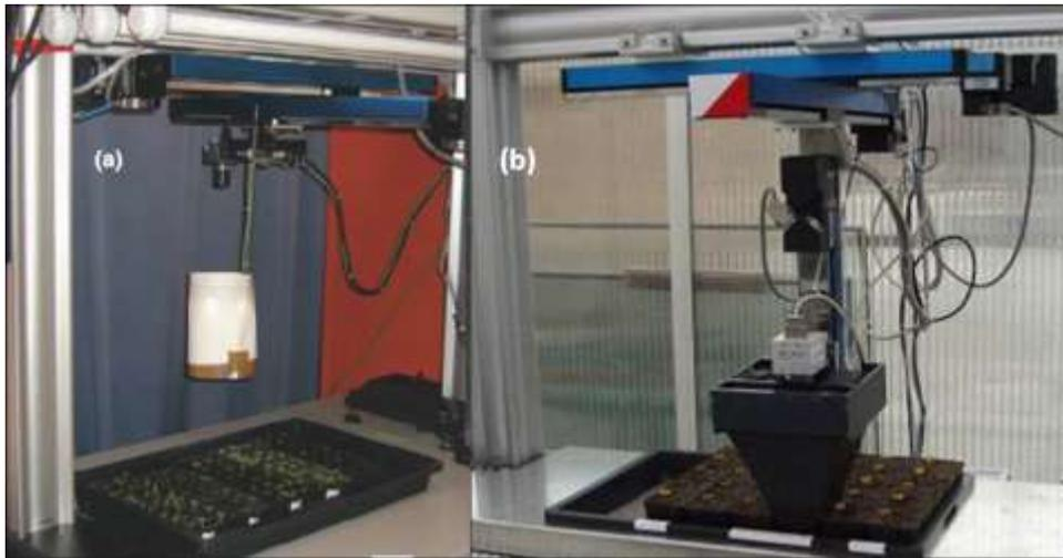
**Figure: 8** Non-invasive leaf growth measurements using (a) GROWSCREEN and (b) GROWSCREEN FLUORO to measure total projected leaf area (a and b) and chlorophyll fluorescence (b).
