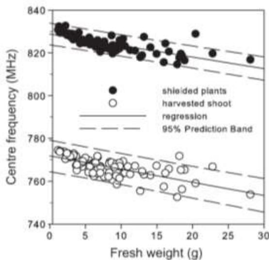
**Figure 7.** Centre frequency offset due to pot shielding in intact plant measurements as compared to harvested shoot measurements. Slope and  $\Delta CF$  not significantly changed.
