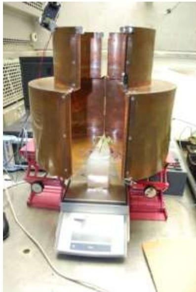
**Figure: 7** View inside the opened folding resonator with a tomato plant grown in agar filled magenta box under enhanced and control UV-B radiation (exposition chambers at Helmholtz Zentrum Munich)
