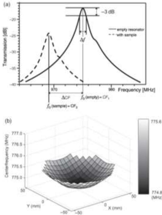
**Figure 2.** Schematics of measurement principle. (a) Transmission curves of microwave resonator P2: empty (solid) and with sample (dashed). Sample causes a relative frequency shift  $\Delta CF = CF_2 - CF_1$ . (b) Spatial variation of first mode centre frequency  $f_0$  of resonator P2 in xy-plane at position  $z = 2.44$  mm, relative to centre of resonator ( $z = 0$ ).
