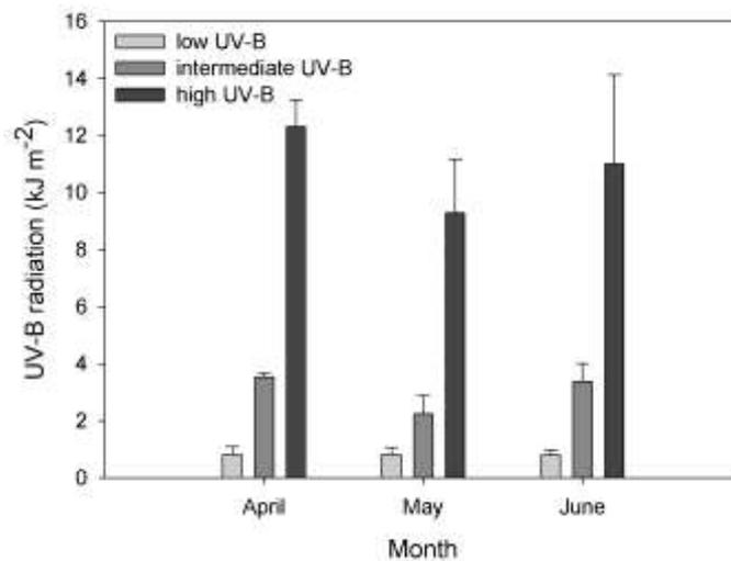
**Figure 2:** Mean UV-B radiation level ( $\text{kJ}\cdot\text{m}^{-2}$ ) transmitted by Float glass (low), MM glass (intermediate) and ETFE foil (high UV-B transmittance) in April, May and June. Radiation was recorded by means of a triple sensor (UV-B, UV-A and PAR) for five days at a frequency of one minute.
