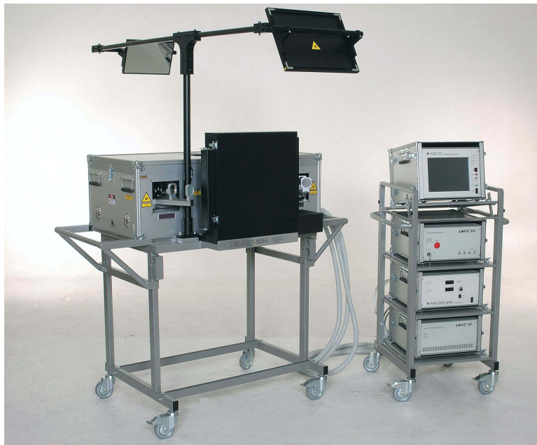
Figure 6.2: Mobile holographic unit HSF-MINI developed together with Geola Uab (Lithuania). The camera is shown without the diffuser plates for eyes-safe operation. The tower on the right houses (from top to bottom) the control unit, the laser power supply, the amplifier power supply and the cooling unit.
