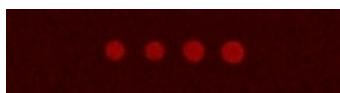
Figure 3.17 Fluorescence image obtained after the hybridization of Cy5 labeled clones from a drinking water biofilm metagenome to the LOV microarray. The image shown corresponds to the probe # 5058 (derived from Novosphingobium aromaticivorans )
