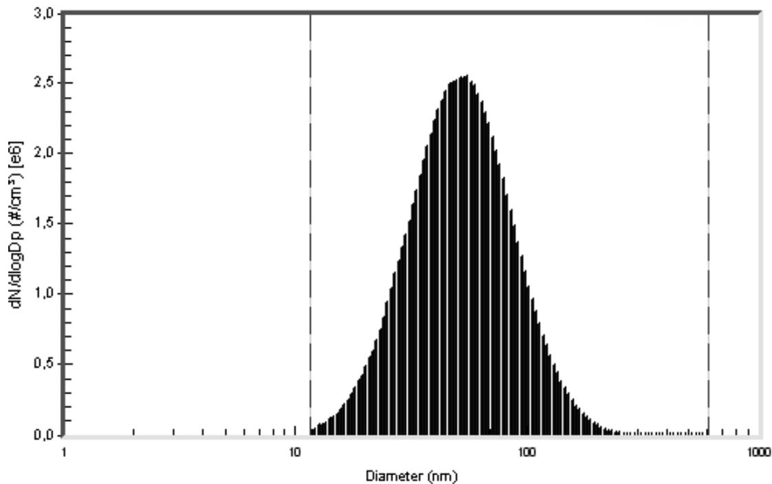
**Figure 1.** Typical size distribution of the carbon nanoparticles generated by the electric spark discharge generator.
