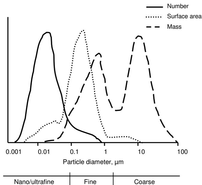
**Figure 1.** Particle size distribution of ambient PM by three characteristics: mass, surface area and number (adapted from Finlayson-Pitts, 2000).
