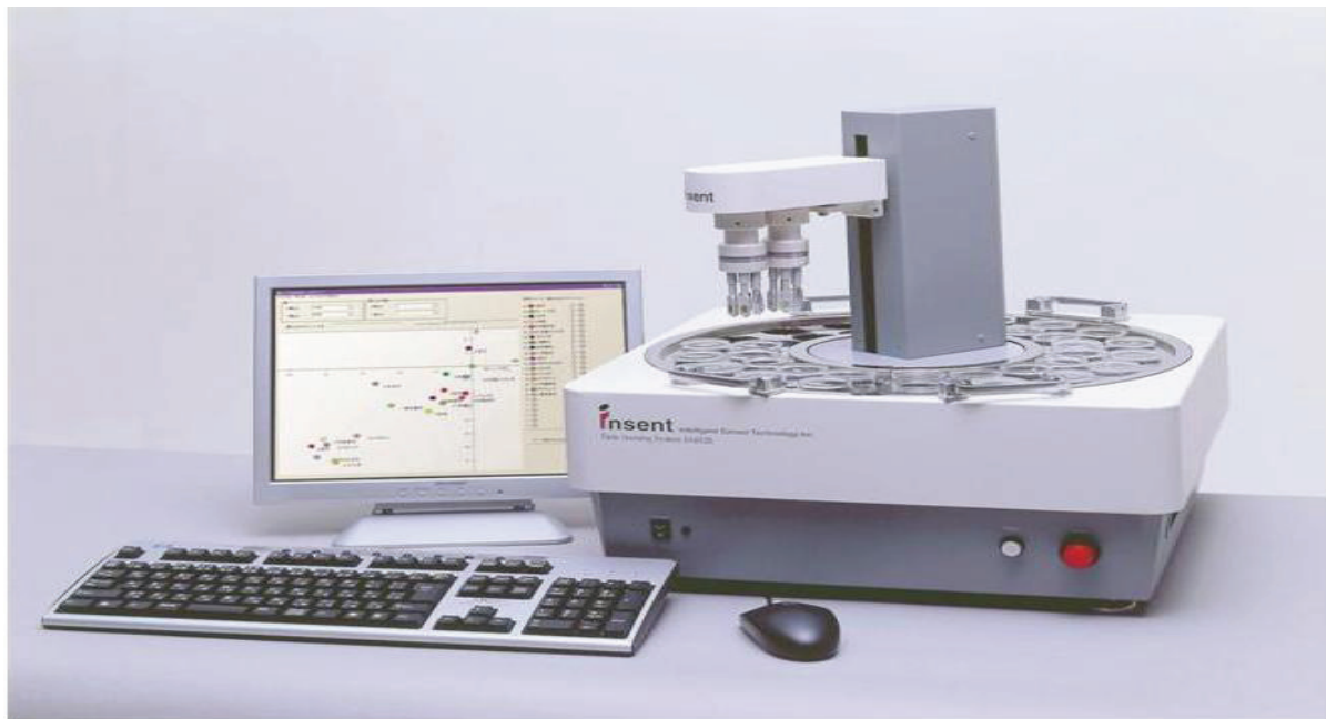
Figure 85: Insent Taste sensing system SA402B, (Intelligent Sensor Technology, Atsugi, Japan).
