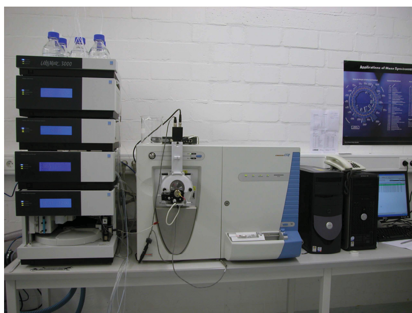
Fig 8: Finnigan LTQ ion trap mass spectrometer (Thermo Finnigan) and HPLC-Ultimate™ 3000 (DIONEX) used in the present study
