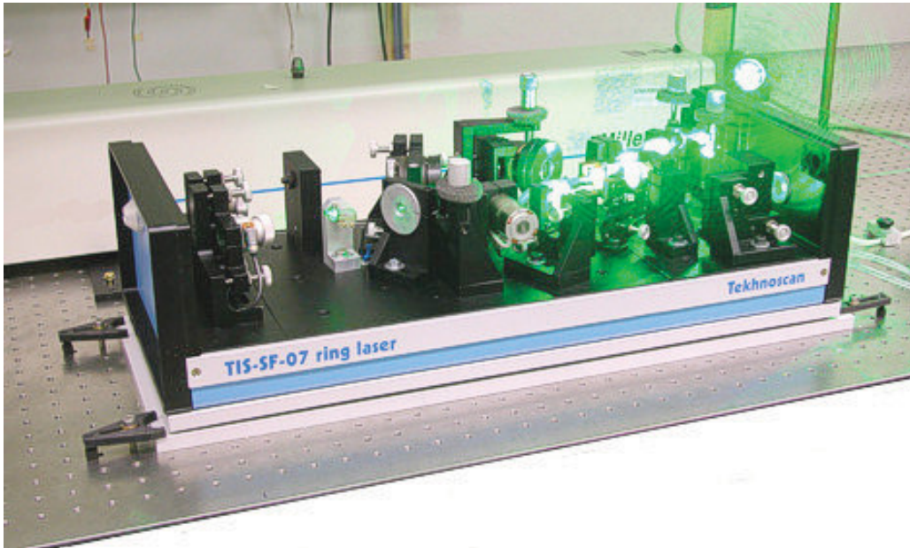
Figure 4.11: Tekhnoscan TIS-SF-07 Titanium-Sapphire laser of the same type as that used as photoassociation laser. (Picture from the company website at http://www.tekhnoscan.ru/english/ )
