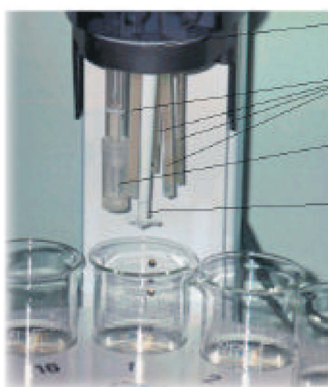
Figure 67: Sensor head with attached sensor array (Alpha-MOS).
