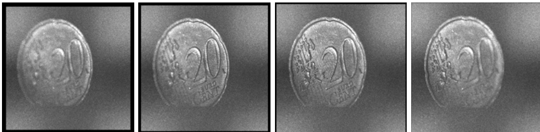
Figure 5.7: Exemplary slices of a scaled image stack, the images closer to the observer are scaled and padded with black. The coin was positioned at 40 cm distance, tilted towards the camera. The inter-slice distance for the examples is 8 mm, a focus progression is visible.
