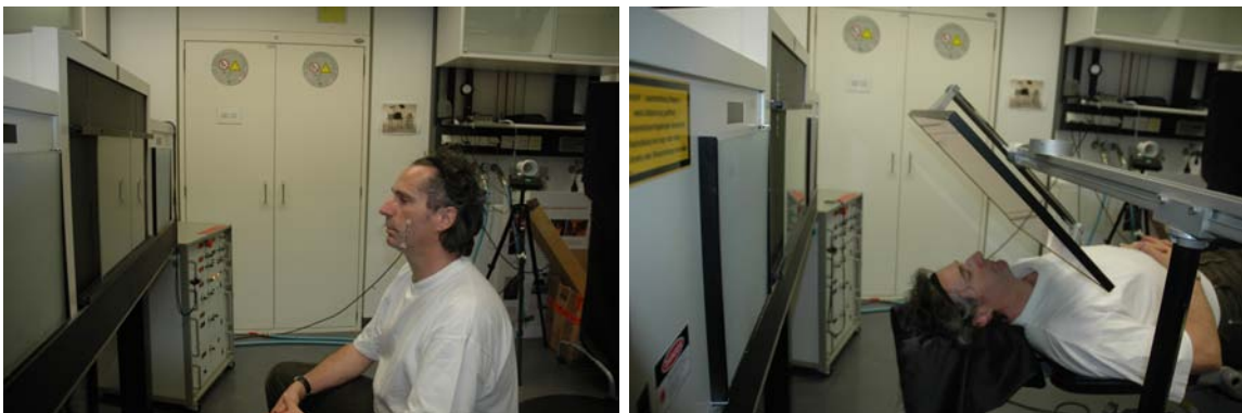
Figure 6.8: Set-up for upright and reclined topometry. The proband wears a jig in each recording.
