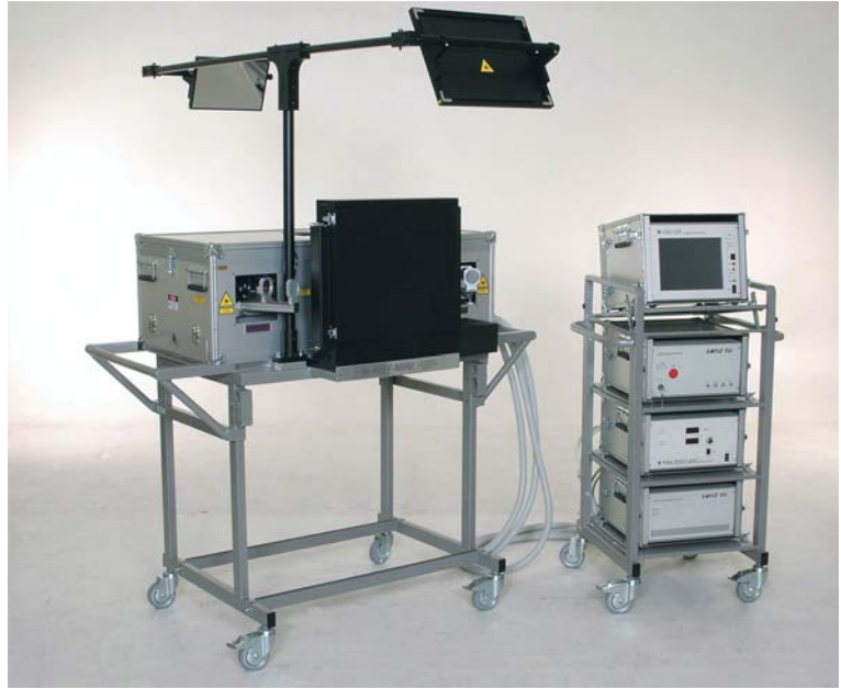
Figure 3.2: Mobile holographic unit HSF-MINI developed together with Geola uab (Lithuania). Here the camera is shown without the diffusor plates for eyes-safe operation. The tower on the right houses (from top to bottom) the control unit, the laser power supply, the amplifier power supply, and the heat exchanger.
