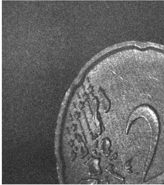
Figure 5.15: Reconstruction of a coin in 40 cm distance from the sensor.
