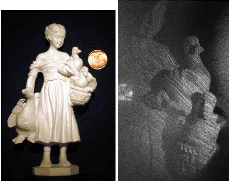
Figure 5.16: A plaster statue shows low texture contrast. The visibility of the surface may be significantly enhanced by the projection of a fringe pattern. Although the object was positioned about 1.4 m from the sensor, a focus progression may be observed.
