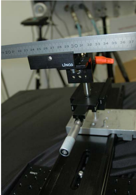
Figure 5.8: A metal ruler is used as a gauging object. With the micrometer screw, the ruler is translated parallel to the optical axis.
