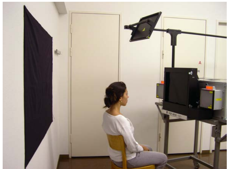
Figure 3.8: Ready for capture. The black shutter curtain covers the hologram plate, so the hologram capture is done in daylight. Left and right are the diffusor plates for eyes-safe recording.
