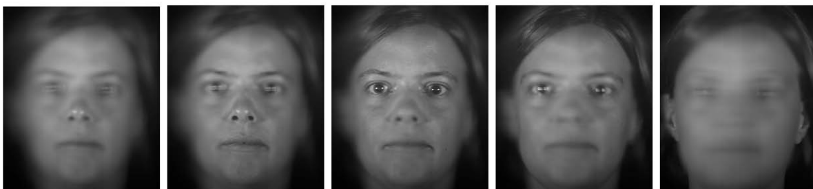
Figure 3.15: Exemplary set of tomograms of the real image at different positions. In each slice some regions of the face are imaged sharply, while others are unfocused. The focus progresses from the tip of the nose up to the ears (from left to right).
