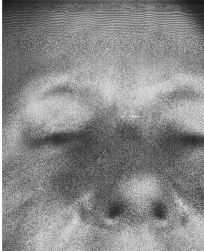
Figure 4.4: Due to height variations of the substrate the flat panel detector shows strong image artifacts. This artifact was eliminated by reducing the height tolerance in the manufacture process.
