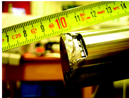
Figure 4.7.1: Electron side of the inner part of the scintillator probe with molten stainless steel
