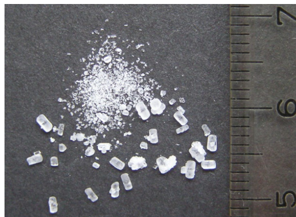
Figure 22: Product crystals of enzyme-assisted PC with 1 mg/mL AArac2440. Grown seed crystals of L-Asn can be distinguished clearly from fine secondary crystals of D- and L-Asn (scale in cm).
